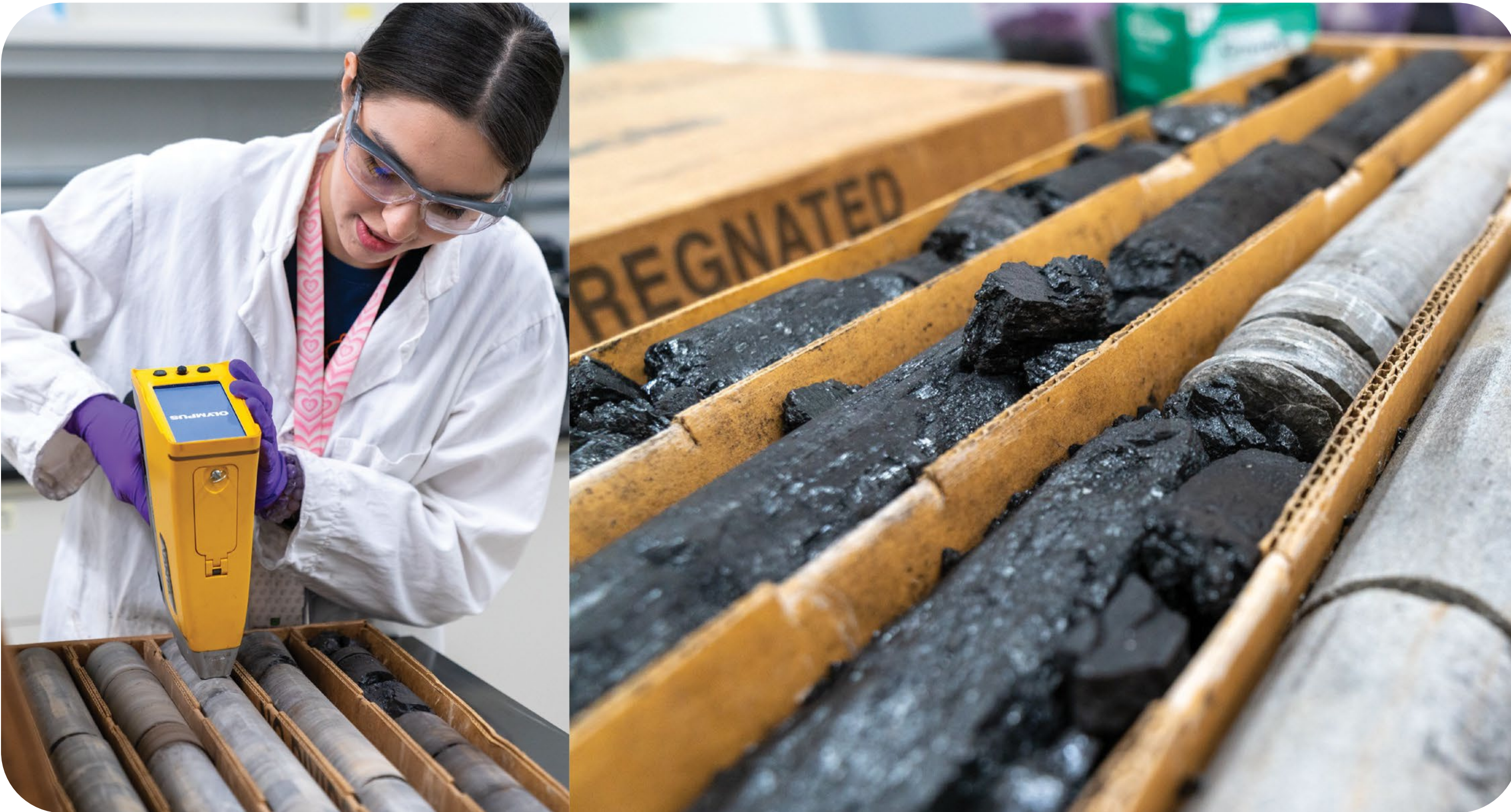
Researcher Obarr examines rock core with a handheld X-ray fluorescent spectrometer.
